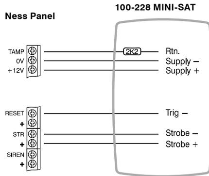
MINI-SAT WIRING TO NESS PANELS
