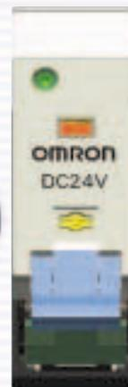
Pull down the test button to the first stop position, then press the yellow button with an insulated tool to operate the contact.
