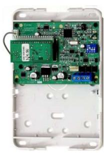
Please Note: For best receiver range ensure the antenna is streched out horizontal from the receiver PCB out the case. Do not mount the receiver inside the M1 housing near the M1 Control panel.
