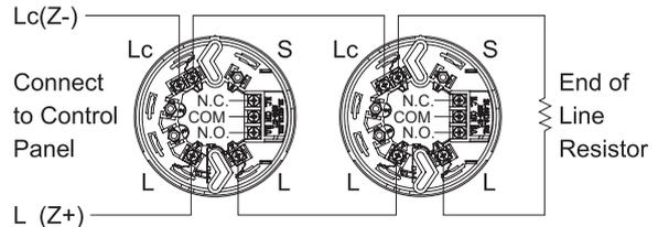
Caution : Do not connect loop wires at same point to prevent function loss.
