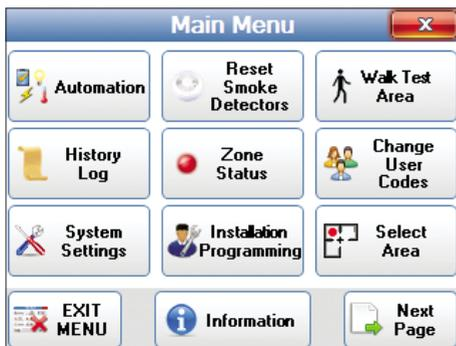
On the Main Screen press "MENU", then press "Next Page" to locate the Synchronise button.
