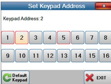
The current keypad address will be highlighted. Addresses with a RED border are already enrolled to the M1 panel and are not available for use.
