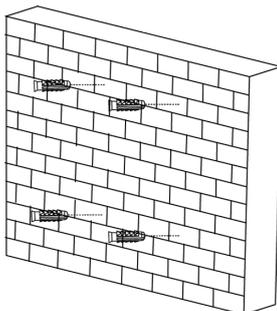
Insert 4 expansion tubes into the wall.
