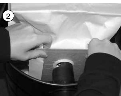
② Remove the full bag by sliding the bag's rubber cuff and collar off the plastic inlet stem (bag adaptor) inside the canister. Once the bag is off the inlet stem, seal the dirt in using the self-adhesive tab provided on the bag's collar. Then lift the paper bag from the dirt canister and dispose in your normal household rubbish bin.
