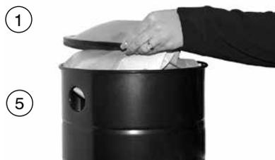
① Remove the lid off the canister by lifting up. There are no hinges or clamps on most power units.
